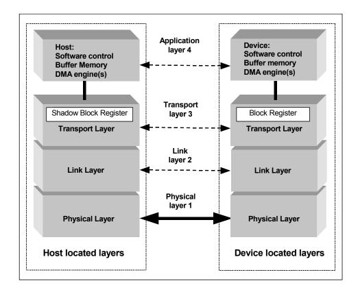
Figure 5.3 Conceptual diagram of communication layers
